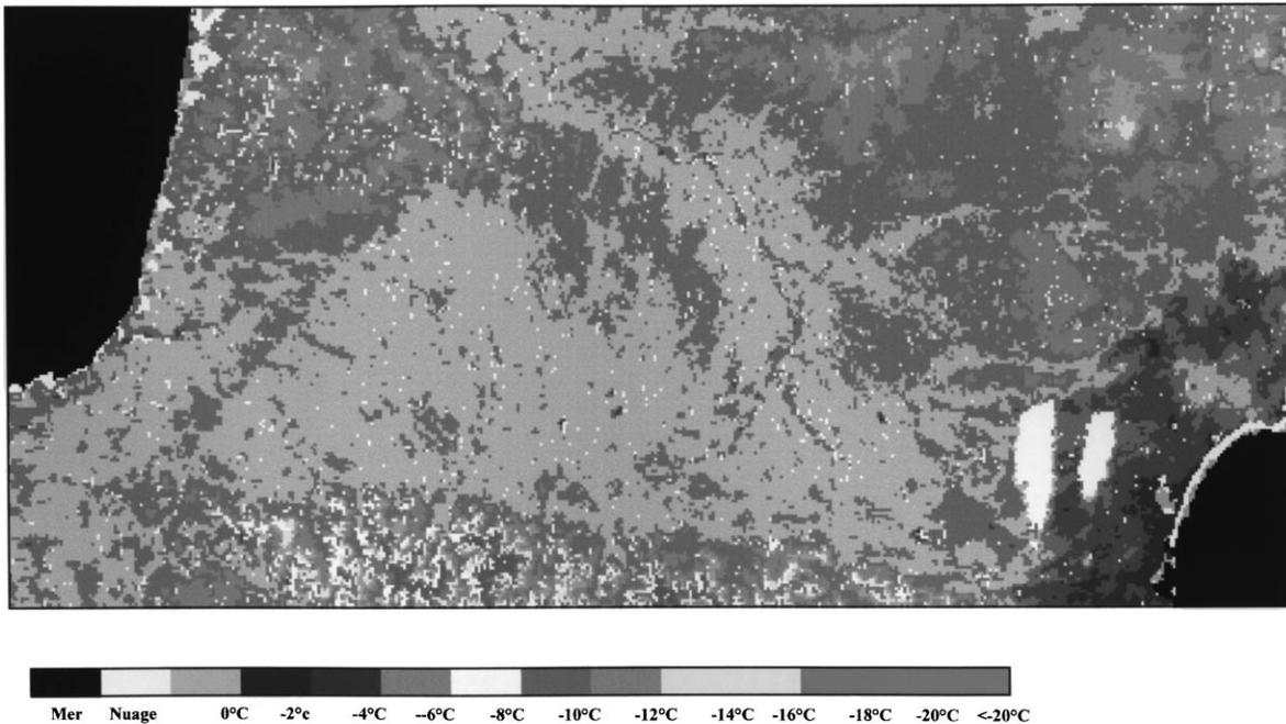
Fig. 6. Surface temperature on 25th February 1993 in the south-west of France. The algorithm used in the calculation is a linear combination of the satellite's AVHRR channels (split-window technique) that enables most atmospheric effects to be eliminated.
