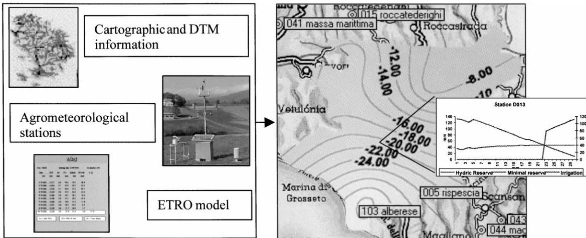
Fig. 4. Water deficit of the Grosseto lowland (26 June 1997) as estimated by ETRO. In input the different informative layers and in output the cartographic representation.
