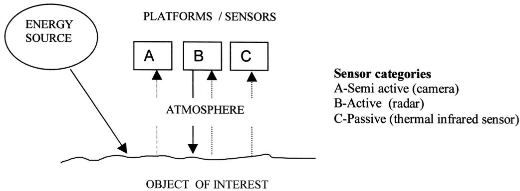
Fig. 5. Main types of remote sensing techniques.
