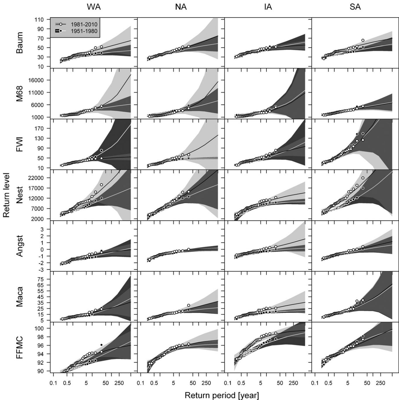
**Fig. 7.** Generalized extreme value return level plots for the different fire danger indices in the 4 regions under consideration. The white line with the black circles refers to the time period 1951–1980, the black line with the white circles to the period 1981–2010. Shading indicates the respective 95% confidence intervals.
